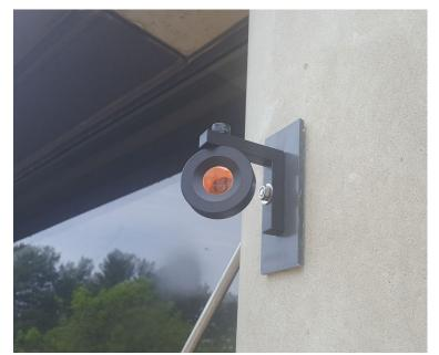
Optical survey target mounted on masonry structure
