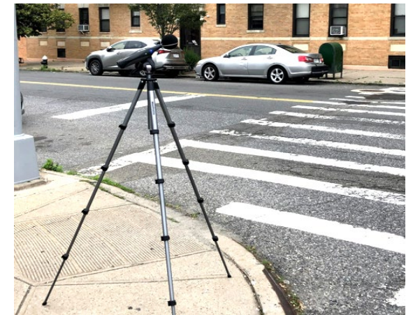
Sound level meter installed outside on sidewalk
