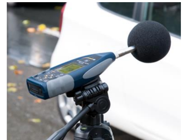
Sound level meter installed outside on sidewalk
