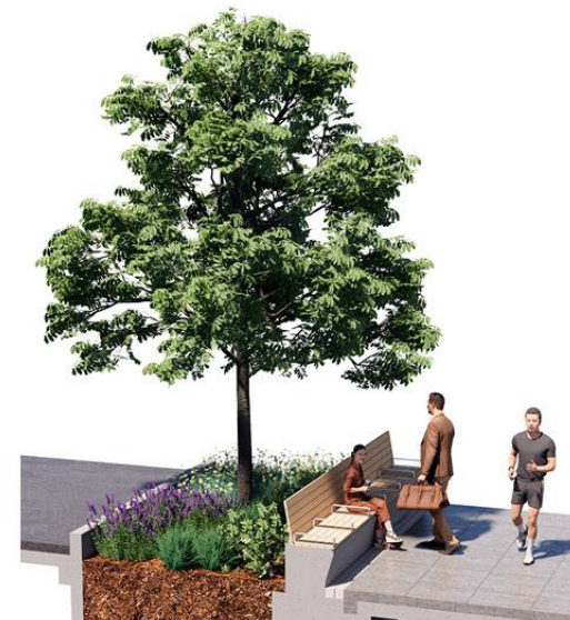
Crash Rated Concrete Seatwall with Planter
