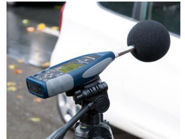
Sound level meter installed outside on sidewalk
