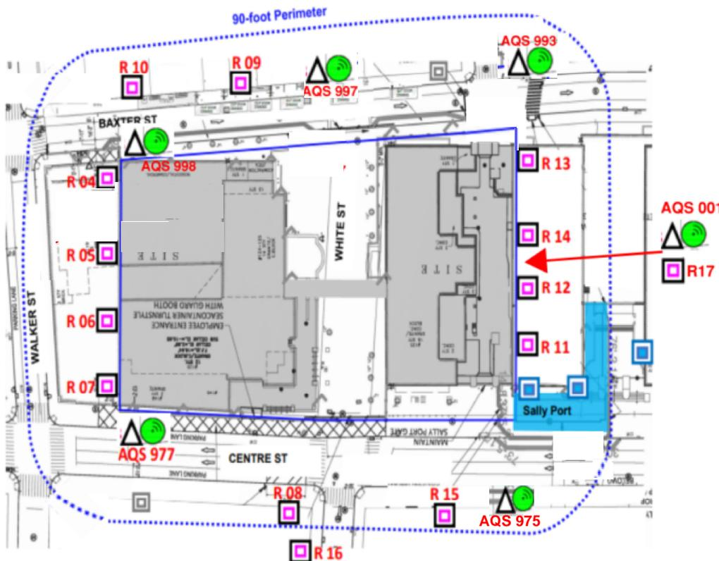
\* Dismantle project vibration, air and noise monitoring devices are installed by Design-Build team in Phase 2, after sally port construction. A vibration monitoring station was installed in the DCTV Fire house at 87 Lafayette St.
