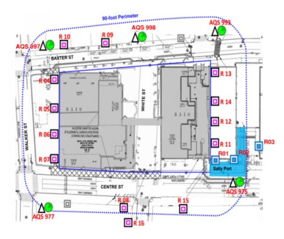
\* Dismantle project vibration, air and noise monitoring devices are installed by Design-Build team in Phase 2, after sally port construction. A vibration monitoring station was installed in the DCTV Fire house at 87 Lafayette St.
