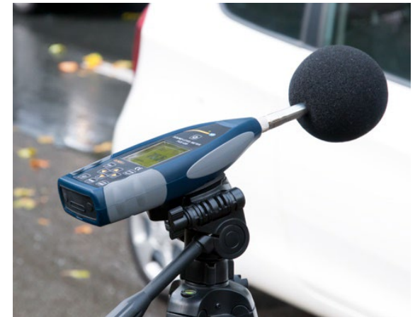
Sound level meter installed outside on sidewalk 安裝在人行道的監測聲音級別儀器
