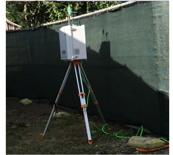
Air Quality monitor installed close to site fence 安裝在工地圍欄附近的空氣質量監測儀
