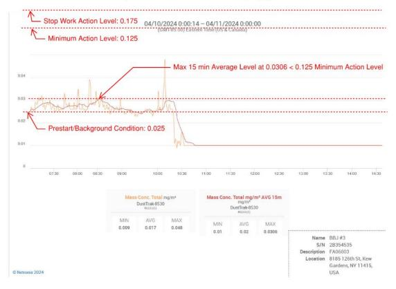
Note: The downwind fixed station recorded constant readings at approximately 1045 due to dust levels near the dust meter's detection limit.
