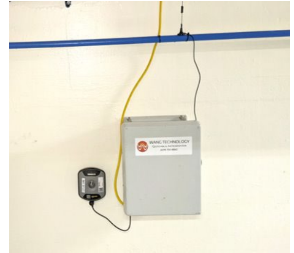
Vibration monitor installed in basement
