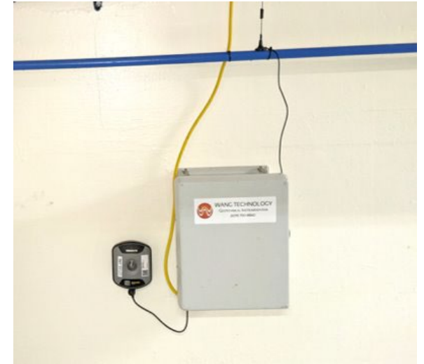
Vibration monitor installed in basement
