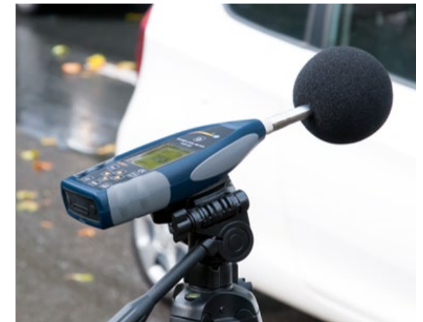
Sound level meter installed outside on sidewalk
